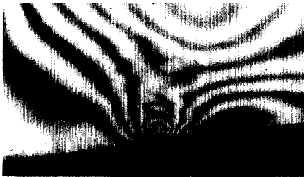
Frame 15: t = 108 \mu\text{s} , a/w = 0.49 , v/c_1 = 0.3
